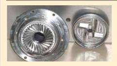
The QuadSlot mixing head is a multistage rotor/stator with a fixed clearance. It is used for applications where very high shear levels are required. The QuadSlot generator produces higher pumping rates and requires higher horsepower than a similar size X-Series rotor/stator set.
