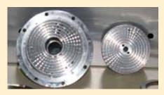
The X-Series head (U.S. patent number 5,632,596) consists of concentric rows of intermeshing teeth. The product enters at the center of the stator and moves outward through radial channels in the rotor/stator teeth. Tolerances are extremely close and the rotor runs at very high tip speeds (typically up
